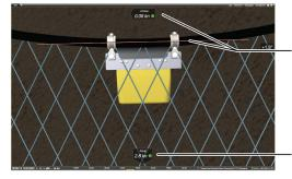
Control if the trawl opening has the correct angle. Across speed needs to be around o.
