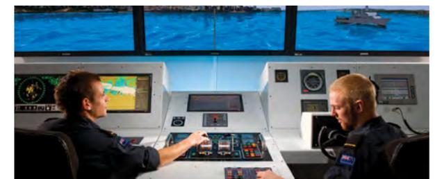
**GMDSS SIMULATOR** imitates ship-to-ship and ship-to-shore communications using simulated terrestrial and satellite communication systems
