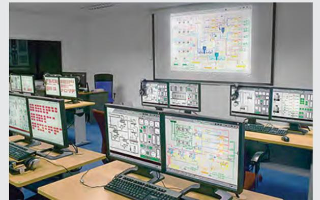
**LIQUID CARGO HANDLING SIMULATOR** enables the training and competence assessment of crew working on liquid cargo tankers, gas carriers and shore terminals, as well as other staff responsible for the safe cargo handling operations and auxiliary equipment
