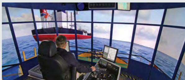
Fully integrated **TUG SIMULATOR** provides users with effective tools for both ship assistant training tasks and professional training in tug and barge operations
