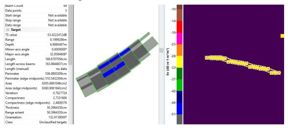
Target properties on left, target on multibeam variable in centre, fish track detected from targets on right.
