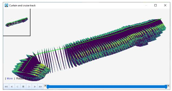
d) Using the Maximum Intensity operator to view "stacked beams", where each sample at range R contains the maximum value of all corresponding multibeam samples that are also at range R, which gives a helpful overview of data throughout the survey.
