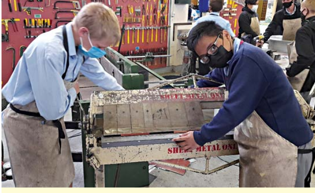
(Pictured above, left and right): Connor Duffell and Ben Ciron using the box and pan folder, used for bending the metal.
