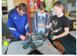
Team one (pictured above) consisting of *Harry Taylor*, *Adam Keen* and *Alec Whitticase* designed a rolling lift bot that could collect three balls and push above the goal bar.
